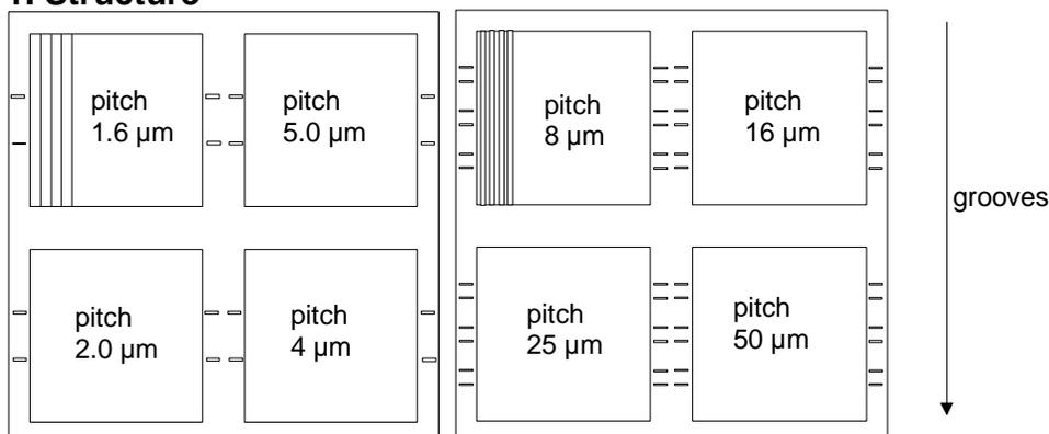
The gratings of type Gr-4P consist of fields of V-grooves. Four fields with a size of 4 mm x 4 mm and different pitch lengths lie inside a chip of 10 mm x 10 mm (thickness of the chip 525 μm). Right and left hand side of these fields there are marks (double lines 300 μm x 30 μm) in positions of 1.5 and 2.5 mm resp. 1, 2 and 3 mm along the grooves. The width of the grooves is approximately equal to the distance between them. These gratings can be used for different applications.
